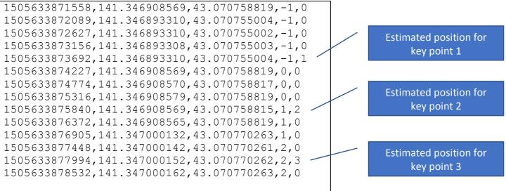
Evaluation will only take into account the estimated position at each indexed key point position, so that each track is considered as a series of key point positions (from 1 to N).
