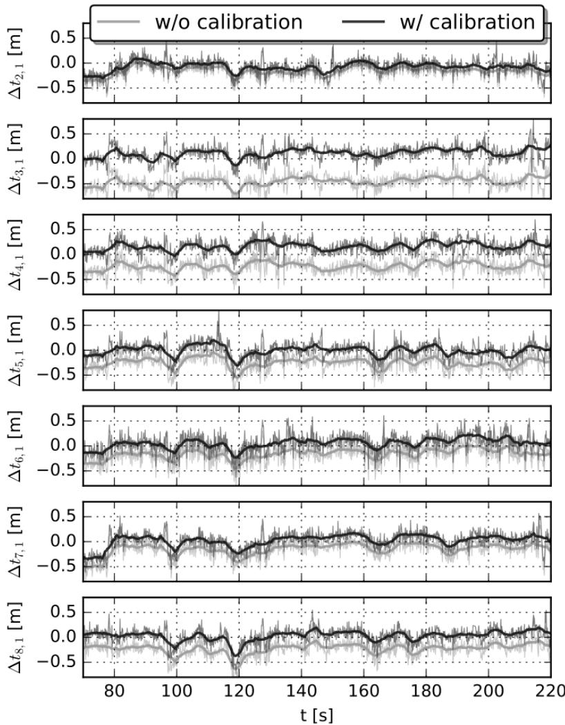
Calibration of static error of each TDOA through node with known position
