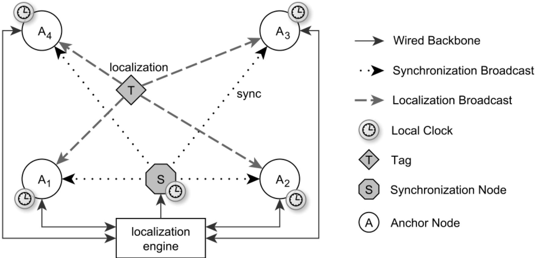
Distributed setup is possible through wireless clock synchronization
