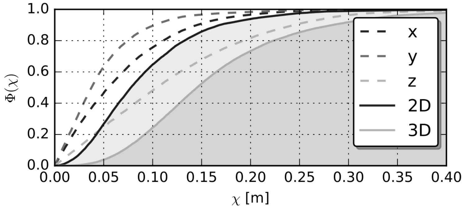
90% Quantile of the horizontal positioning error in the range of ~20cm
