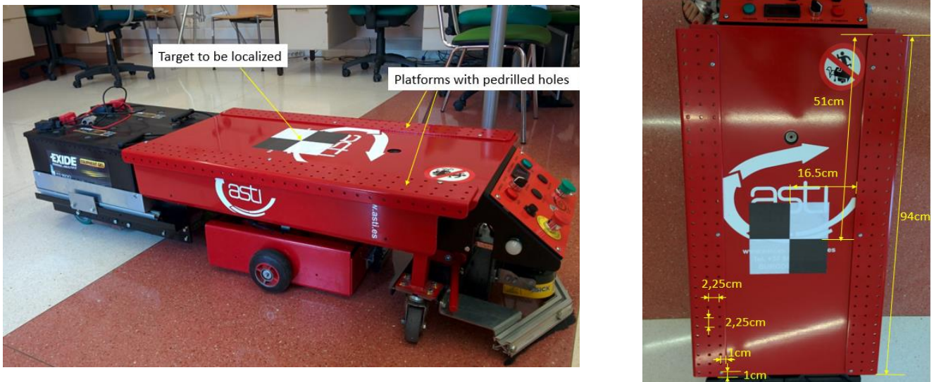
Figure 5. Photo of the robot, including the predrilled platform and the pattern that indicates the reference point to be localized.
